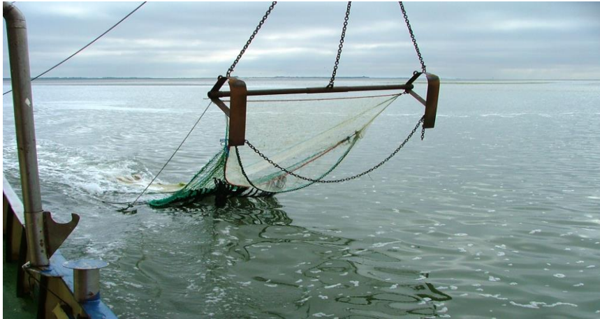
Fig. 1. Beam trawl, (1) - http://iara.government.bg/wp-content/uploads/2013/08/Biim-tral.jpg , (2) - https://www.maritime.bg/wp-content/uploads/2013/08/biim-tral.jpg .
